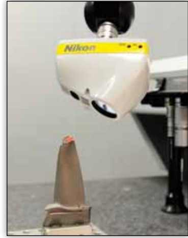
Turbine blades Eliminate probe tip compensation errors
