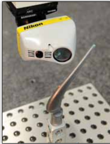
Medical implants Inspect complex freeform geometry
