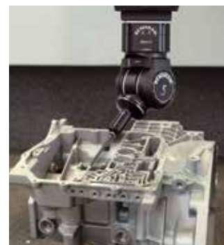
REVO-2 5-axis measurement system
